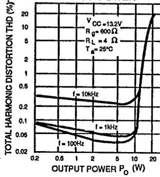
Fig. 4 - TOTAL HARMONIC DISTORTION vs. OUTPUT POWER
