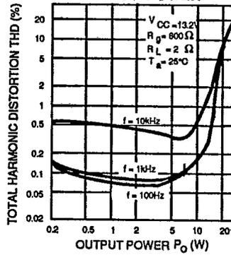
Fig. 5 - TOTAL HARMONIC DISTORTION vs. FREQUENCY
