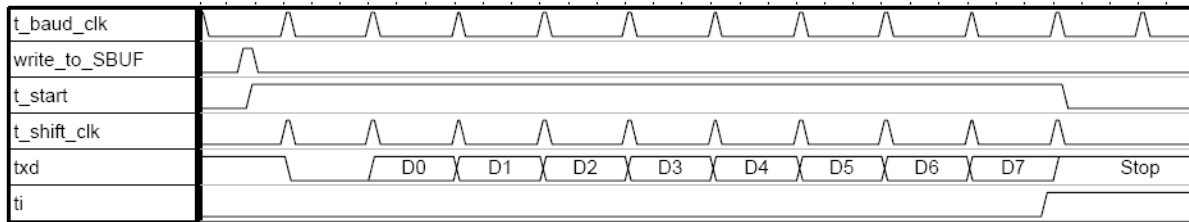
Fig. 7-3: Transmit mode 1 for Serial 0
