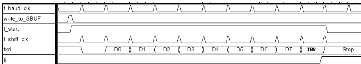
Fig. 7-5: Transmit modes 2 and 3 for Serial 0
