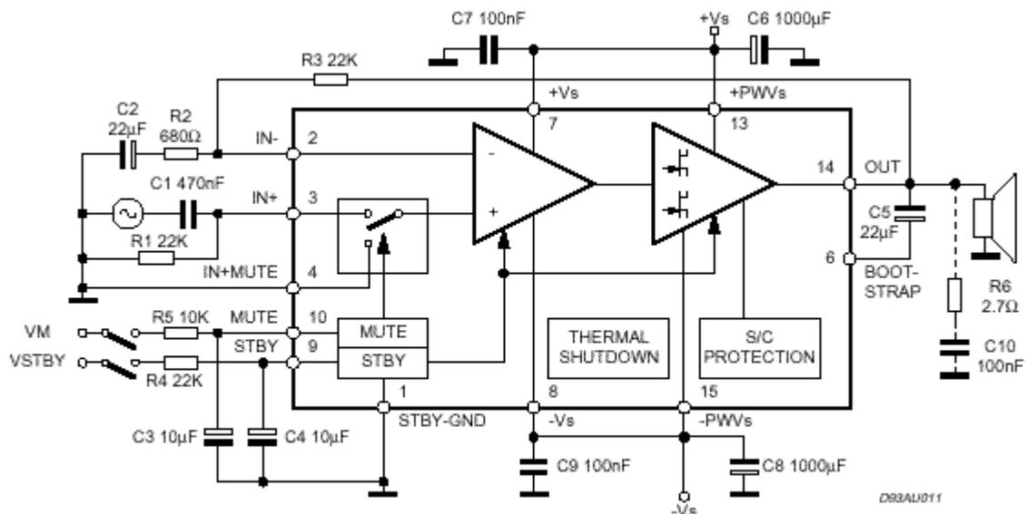
Note: The Boucherot cell R6, C10, normally not necessary for a stable operation it could be needed in presence of particular load impedances at  $V_{CC} < \pm 25V$ .
