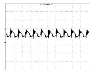
**Figure 11:** Input Terminal Ripple Current,  $i_c$ , at full rated output current and nominal input voltage with 12µH source impedance and 33µF electrolytic capacitor (200 mA/div, 2us/div).
