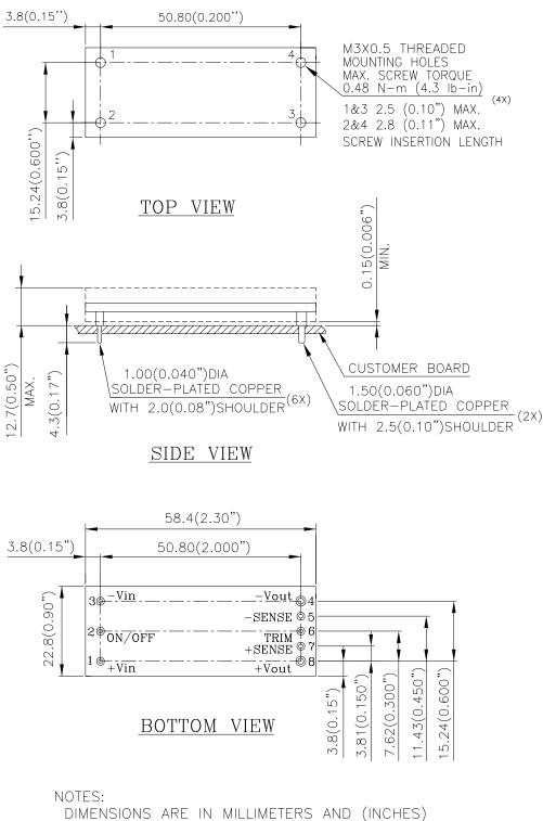
DIMENSIONS ARE IN MILLIMETERS AND (INCHES) TOLERANCES: X.Xmm±0.5mm(X.XX in.±0.02 in.) X.XXmm±0.25mm(X.XXX in.±0.010 in.)
