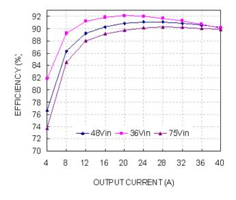
Figure 1: Efficiency vs. load current for minimum, nominal, and maximum input voltage at  $25^{\circ}$ C
