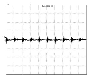
**Figure 12:** Input reflected ripple current,  $i_s$ , through a 12µH source inductor at nominal input voltage and rated load current (20 mA/div, 2us/div).
