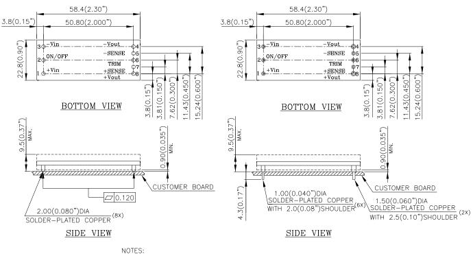
DIMENSIONS ARE IN MILLIMETERS AND (INCHES) TOLERANCES: X.Xmm±0.5mm(X.XX in.±0.02 in.) X.XXmm±0.25mm(X.XXX in.±0.010 in.)
