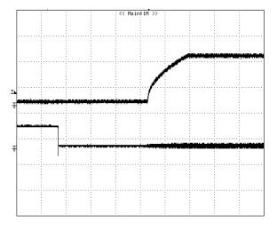
*Figure 4:* Turn-on transient at zero load current (2 ms/div). Vin=48V.Top Trace: Vout, 1V/div; Bottom Trace: ON/OFF input, 5V/div *Figure 5:* Turn-on transient at full rated load current (constant current load) (2 ms/div). Vin=48V.Top Trace: Vout, 1V/div; Bottom Trace: ON/OFF input, 5V/div
