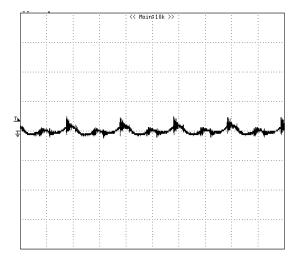
**Figure 14:** Output voltage ripple at nominal input voltage and rated load current (Io=40A)(20 mV/div, 2us/div)
