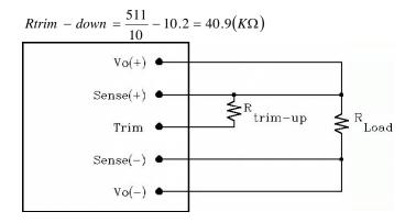
*Figure 19:* Circuit configuration for trim-up (increase output voltage)
