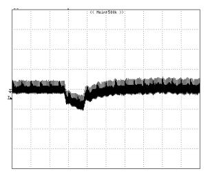
**Figure 8:** Output voltage response to step-change in load current (75%-50% of lo, max; di/dt =  $0.1A/\mu$ s). Load cap:  $10\mu$ F, tantalum capacitor and  $1\mu$ F ceramic capacitor. Trace: Vout (20mV/div, 100us/div), Scope measurement should be made using a BNC cable (length shorter than 20 inches). Position the load between 51 mm to 76 mm (2 inches to 3 inches) from the module..
