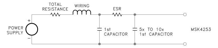
Be careful of the ripple current in all the capacitors. Excessive ripple current, beyond what the capacitors can handle, will destroy the capacitors.
