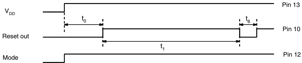
Figure 4. Power-up Reset and Mode Switchover
